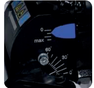
Continuous angle adjustment from 0 to 60 degrees.
