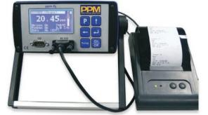
Connecting a printer via the RS232 interface. Capable of readout documentation (per second) that can be logged via a printer.
