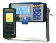
Connected via a Bluetooth Dongle with a range of up to 100m to a mobile phone.
